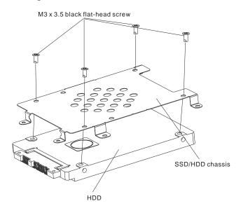
Figure 4-13 Removing the SSD/HDD chassis
